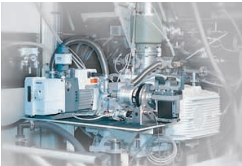
Leak detection system
